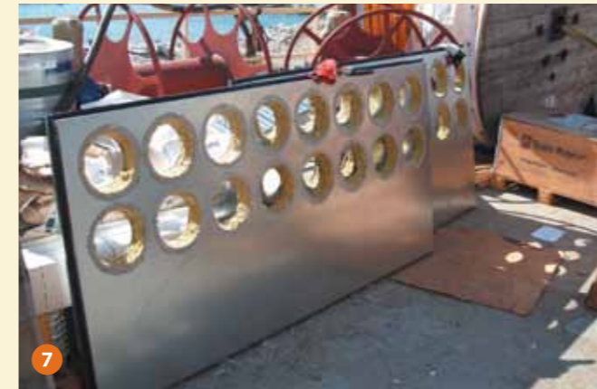
The holes for spiro pipes can be taken on site to fit 100% with the spiro pipe system.
